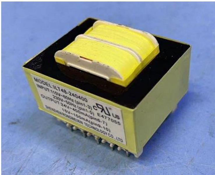
Photo 16 - Unlisted Component Transformer ILT48-240400.
